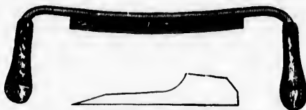
No. 1. Section of Blade, Full Size.
